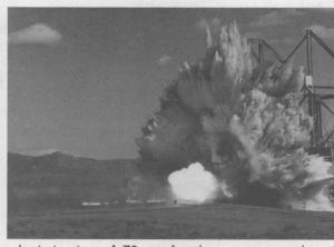
GOING, GOING, GONE — Sequence shows rocket sled test of F-4 Phantom jet aircraft as it slams into a one-million-pound block of concrete. The first-of-its-kind test was designed to help researchers estimate the effect of an aircraft crashing
